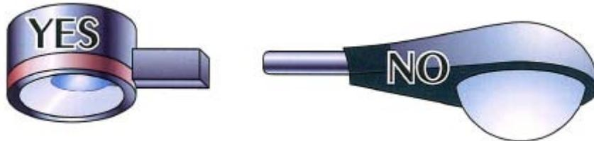
Same fixture as above, mounted incorrectly defeating the horizontal mounting design. The fixture now produces direct glare and can also produce upward thrown light, sometimes at steep mounting angles.
