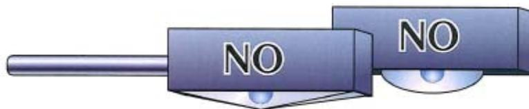
Forward-Throw Style. Exposed bulb in forward direction produces some direct glare.
