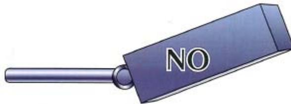
Known as "cut off," center drop or sag lens with or without exposed bulbs still produces direct glare.
